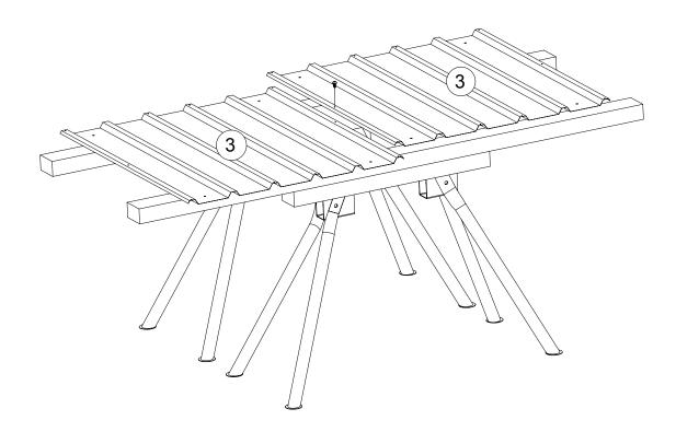
Now tap or slide 2 x part 20A (channels) onto the sheeting and fix them to the top and bottom with self-tapping screws. Make sure that the small lips on channels 20A are always facing out. This ensures rainwater cannot build up inside your shed.
