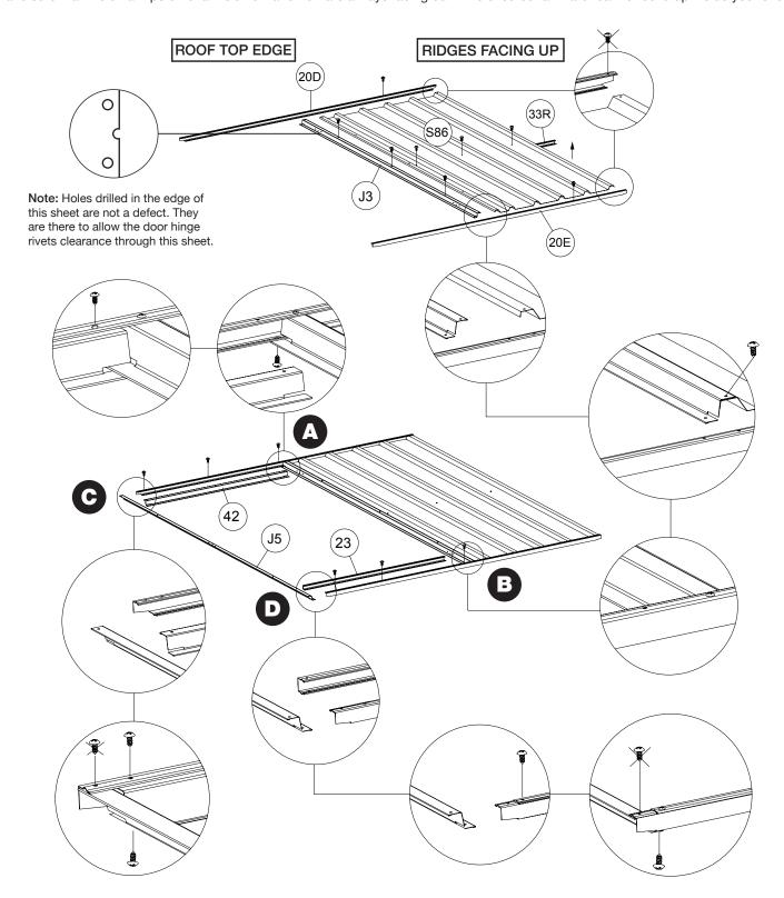
Fit part J5 (jamb), part 42 (jamb) and part 23 (bottom channel) and fix them with self-tapping screws - except those marked with a cross. Make sure both joins (diagrams A and B) are fixed the same followed by diagrams C and D.
